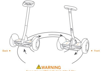
Always step on/off from the back of the S-Max. Otherwise you risk falls and/or collisions because the steering direction is reversed.
