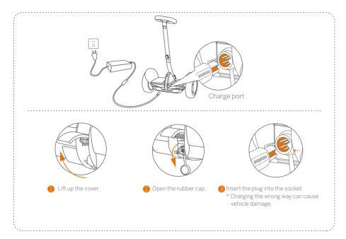
Your S-Max is fully charged when the LED on the charger changes from red (charging) to green (trickle charge).
