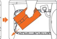
Apply a little pressure to the center of the plastic rivets with a screwdriver of sharp-pointed tool to loosen them up. Pull them out and remove the
